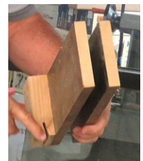
Angled Spline Saddle Jig
