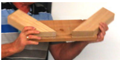
Corner Spline Jig
