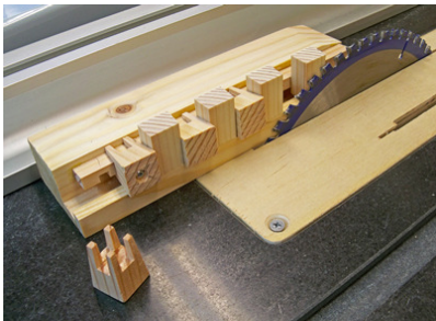
Rough trimming the legs on the table saw
