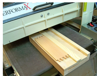
Using the fixture for drum sanding
