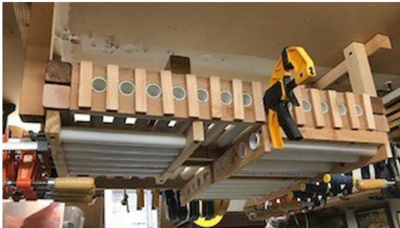
As a further enhancement of the original design, he installed vertical slats between the tubes to hold the clamp heads upright, keeping them from flopping over and getting tangled – great idea, **Don!**
