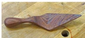
In addition, **Tom** also brought along a couple more of his recent creations. The first was a wooden spatula, that he explained was made with a 2D bandsawing technique in which the piece is sawn from a block face up and then rotated 90° and resawn to shape on edge. After sanding and smoothing, the lovely Jatoba spatula looked too pretty to use!
