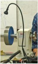
The diamond grinding wheel she uses is an 8” diameter rigid aluminum wheel with fine diamond grit bonded to its outer surface. A custom insert adapted the wheel to the headstock of her lathe. Although somewhat expensive, this tool does an excellent job and has a long anticipated service life – definitely a worthwhile investment for the serious wood turner!
