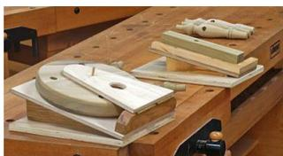
Having established the desired angles for the holes for the spindles and the stretchers, she made a simple double-ended template with one of the angles on each end. She used that template to develop a pair of drill jigs which could be used on her drill press to accurately drill the holes in the seat and the spindle blanks using a Forstner bit.
