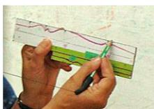
that a story stick is much easier to use and more foolproof than measurements and gives a graphical representation of the desired profile. Though she didn't mention it, I suspect that critical dimensions such as the tenon diameters were noted on the story stick.
