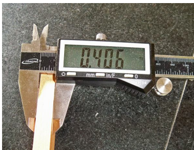
Verifying Spacer Thickness
