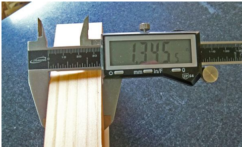
Verifying Stock Blank Thickness
